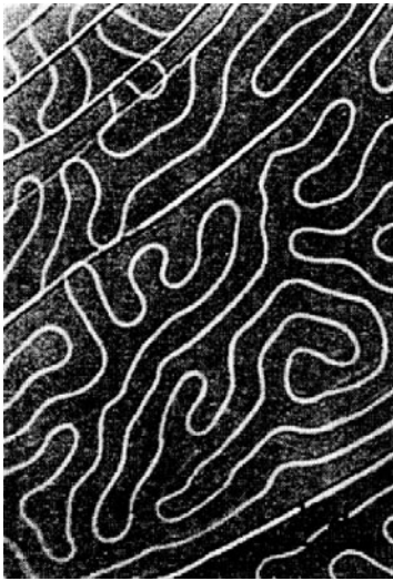
Fig. 16.7 Barium ferrite 180^\circ domains viewed along the hexagonal c -axis. Colloidal suspensions of magnetite particles make the domain walls visible.
